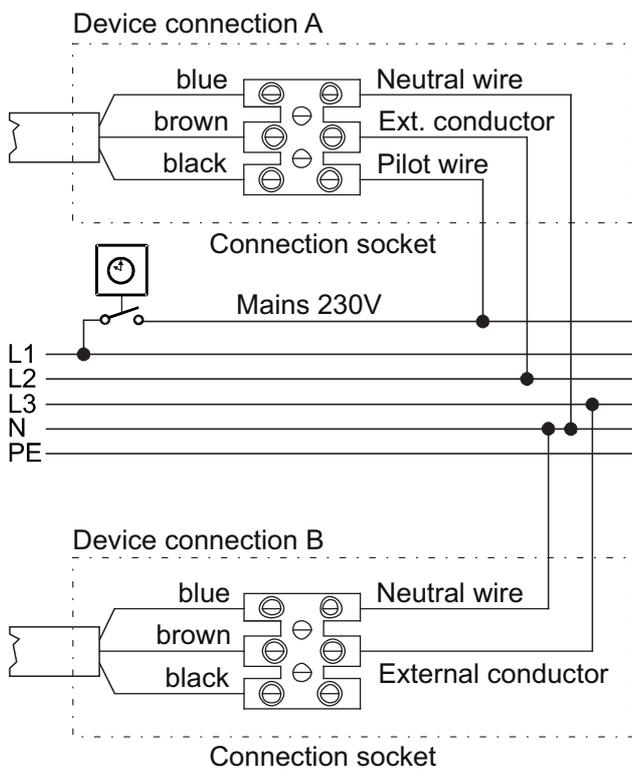
If the black wire is not used, it must be connected to an electrically insulated terminal and not to the power supply.
