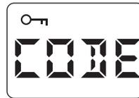
Press the  $\oplus$  and  $\ominus$  keys simultaneously for 3 s until **CODE** flashes.
