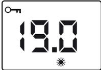
Press the  $\oplus$  and  $\ominus$  keys simultaneously for 3 s until **CLEF 1** and the symbol
