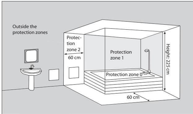
The device can be installed in protection zone 2 or outside of protection zones.
