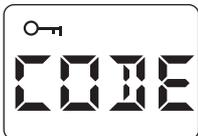
Press the  $\oplus$  and  $\ominus$  keys simultaneously for 10 s until **CODE** is displayed.
