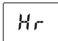
Use the keys  $\oplus$  or  $\ominus$  to select **Hr** and confirm with the  $\text{Mode}$  key.
